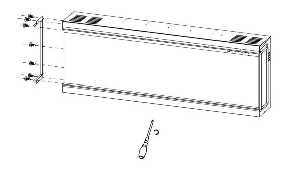
4. Remove the screws from the fireplace as shown in the picture below.
