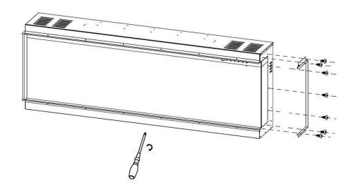
4. Remove the screws from the fireplace as shown in the picture below.
