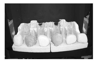
d) Fit pebbles A, B, C, & D behind the ceramic front rails as shown below in Fig. 12 (Pebble markings stamped into bottom face)
