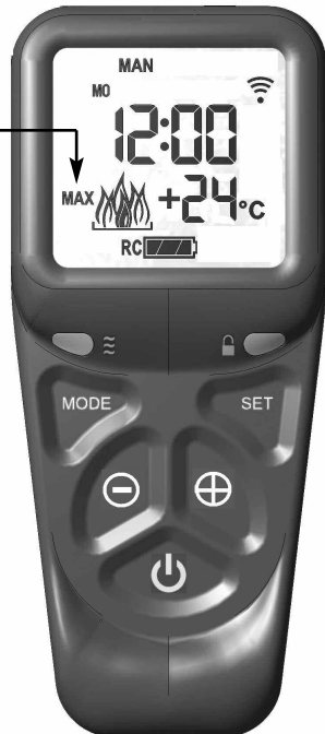
Fig. 3 - "MAX" & large flame symbol displayed
