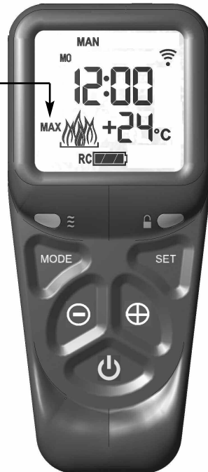
Fig. 41 - "MAX" & large flame symbol displayed
