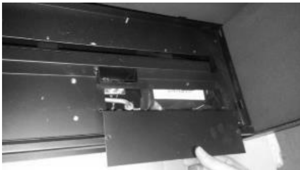
Fig 1. Carefully lift the the ceramic base boards to reveal the burner screws
