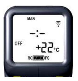
Note: the indicator at the bottom shows the battery condition of both the batteries in the hand set and in the fire control within the fire.
