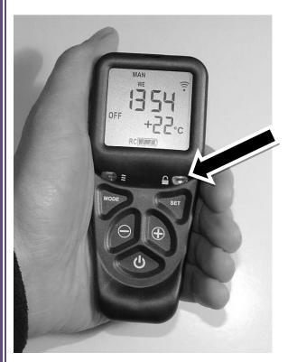
**3)** Setting the time the display will be as shown, as the time is not set yet and will progress automatically to the next screen shown below.
