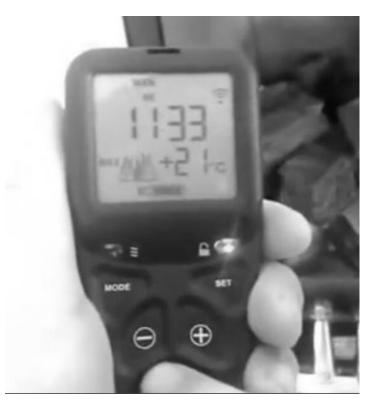
To stop the fire, hold handset to unlock the buttons and then press the power button.
