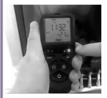
Hold the handset and the green unlock light will illuminate allowing the buttons to work.
