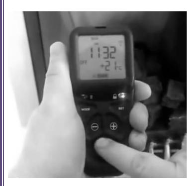
Press and hold in the power symbol button and release immediately when the word pilot appears at the bottom left of the display (after about 1-2 seconds). The fire will light.
