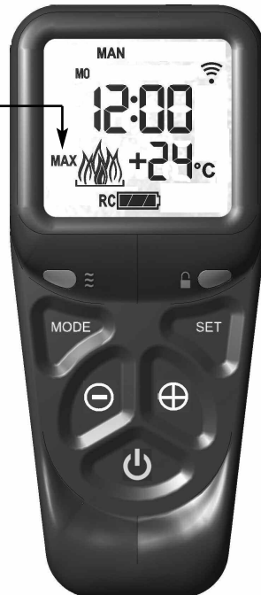
Fig. 3 - "MAX" & large flame symbol displayed
